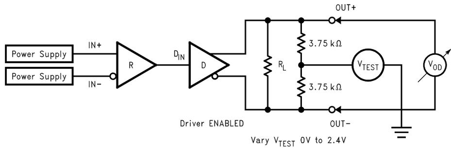
FIGURE 2. Differential Driver Full Load DC Test Circuit
