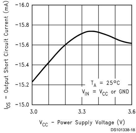
**Differential Output Short Circuit Current vs Power Supply Voltage**
