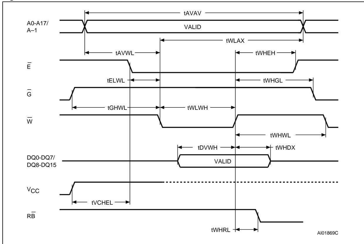
**Table 16. Write AC Characteristics, Chip Enable Controlled**
