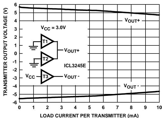
FIGURE 11. TRANSMITTER OUTPUT VOLTAGE vs LOAD CURRENT (PER TRANSMITTER, i.e., DOUBLE CURRENT AXIS FOR TOTAL V<sub>OUT+</sub> CURRENT)
