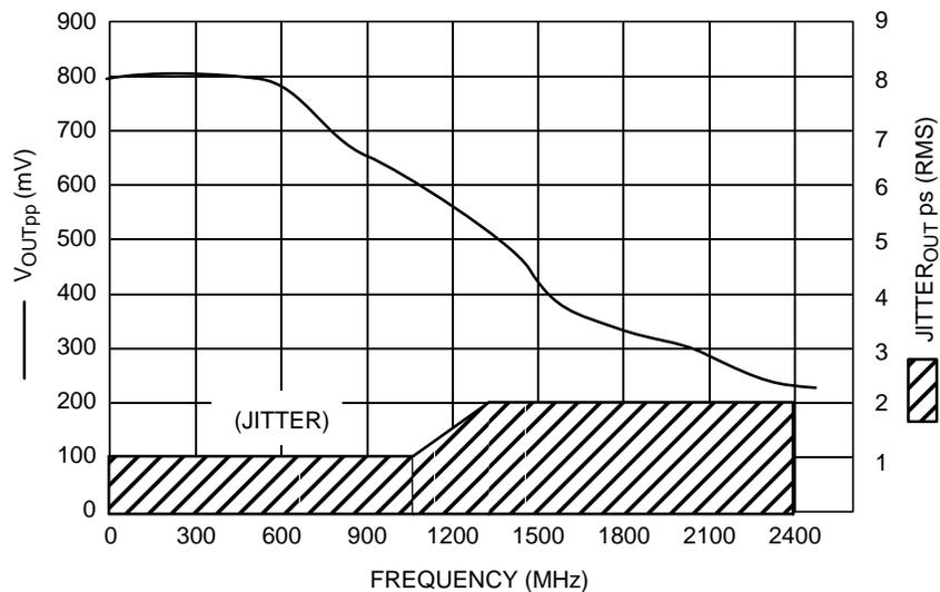
Figure 6. F<sub>max</sub>/Jitter
