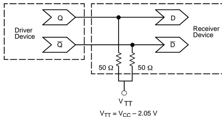
Figure 7. Typical Termination for Output Driver and Device Evaluation
