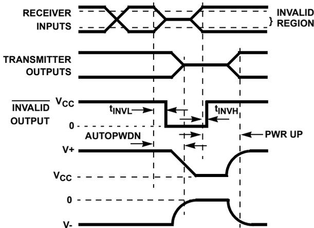
FIGURE 7. AUTOMATIC POWERDOWN AND INVALID TIMING DIAGRAMS
