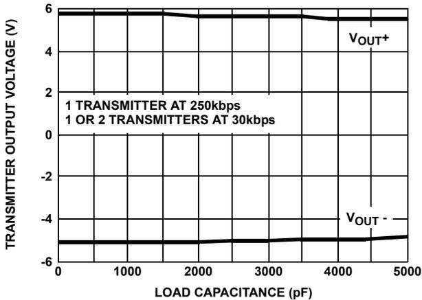
**FIGURE 13. TRANSMITTER OUTPUT VOLTAGE vs LOAD CAPACITANCE**
