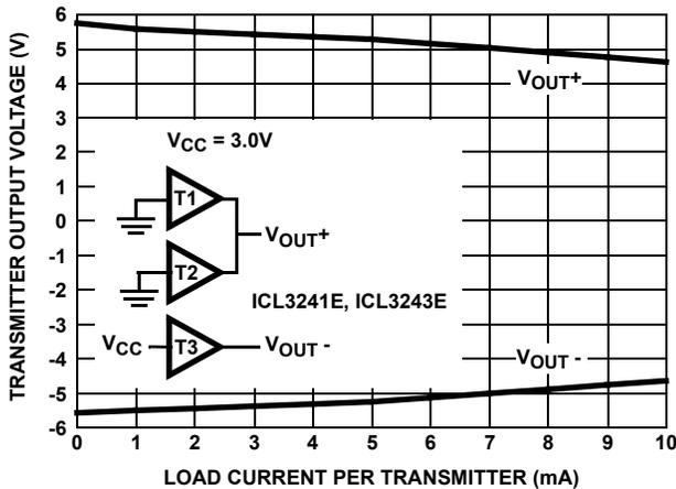
FIGURE 9. TRANSMITTER OUTPUT VOLTAGE vs LOAD CURRENT (PER TRANSMITTER, i.e., DOUBLE CURRENT AXIS FOR TOTAL V<sub>OUT+</sub> CURRENT)
