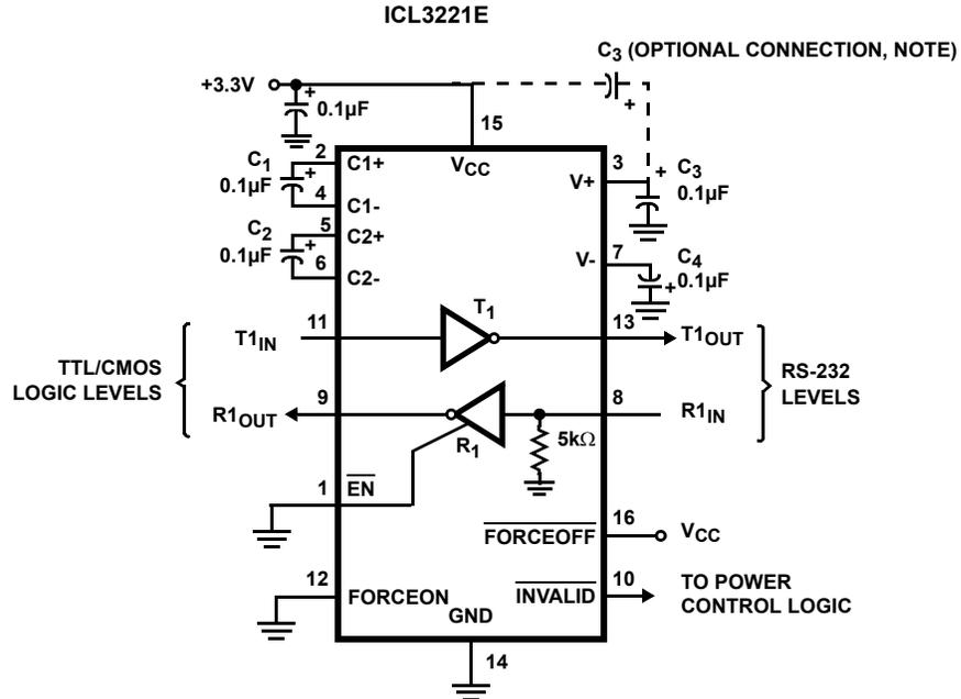
NOTE: The negative terminal of C<sub>3</sub> can be connected to either V<sub>CC</sub> or GND
