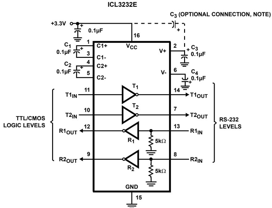
NOTE: The negative terminal of C<sub>3</sub> can be connected to either V<sub>CC</sub> or GND
