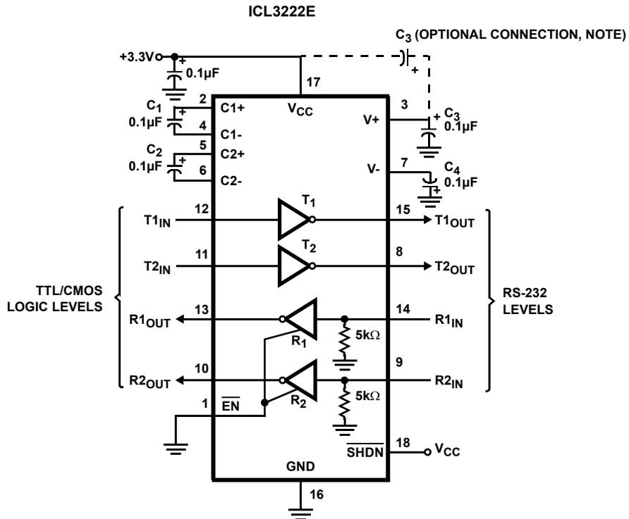
NOTE: The negative terminal of C<sub>3</sub> can be connected to either V<sub>CC</sub> or GND
