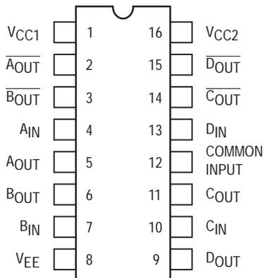
Pin assignment is for Dual-in-Line Package.
