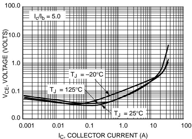
Figure 3. Typical Collector-Emitter Saturation Voltage,  $I_C/I_B = 5.0$
