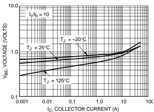
Figure 6. Typical Base-Emitter Saturation Voltage,  $I_C/I_B = 10$
