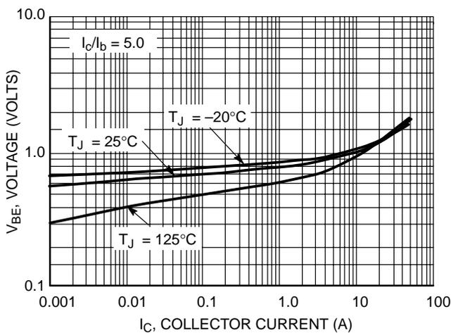
Figure 5. Typical Base-Emitter Saturation Voltage,  $I_C/I_B = 5.0$
