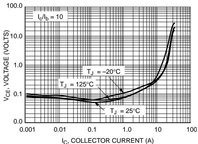
Figure 4. Typical Collector-Emitter Saturation Voltage,  $I_C/I_B = 10$
