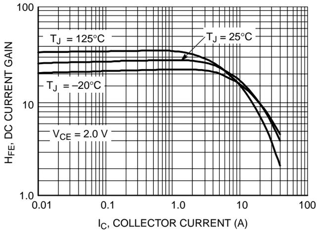
Figure 1. DC Current Gain,  $V_{CE} = 2.0\text{ V}$
