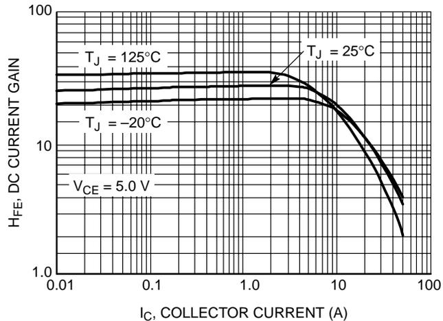
Figure 2. DC Current Gain,  $V_{CE} = 5.0\text{ V}$
