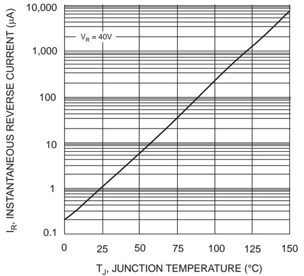
Fig. 4 Typical Reverse Current vs. Junction Temperature
