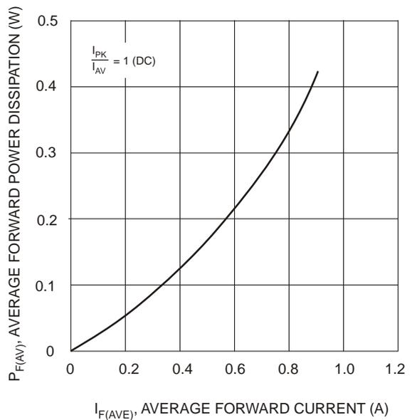
Fig. 6 Forward Power Derating
