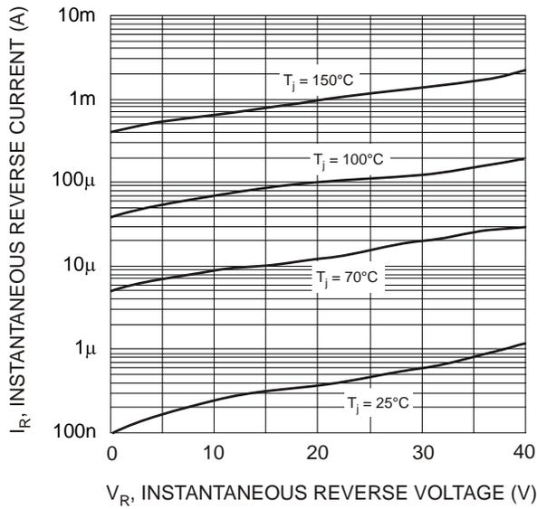
Fig. 3 Typical Reverse Current vs. Reverse Voltage
