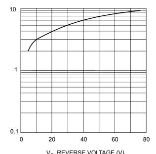
IR, LEAKAGE CURRENT (nA)
