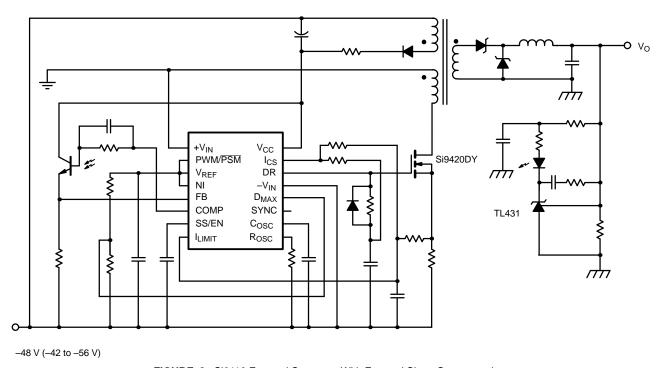
FIGURE 3. Si9119 Forward Converter With External Slope Compensation
