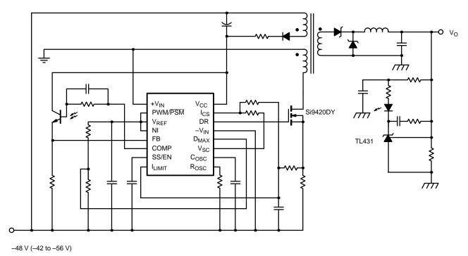
FIGURE 2. Si9118 15-W Forward Converter Schematic
