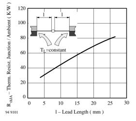
Figure 1. Typ. Thermal Resistance vs. Lead Length
