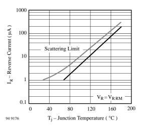
Figure 4. Reverse Current vs. Junction Temperature
