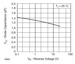
Figure 6. Capacitance vs. Reverse Voltage
