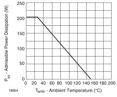
Figure 3. Admissible Power Dissipation vs. Ambient Temperature
