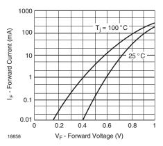
Figure 1. Forward Current vs. Forward Voltage
