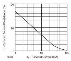
Figure 4. Dynamic Forward Resistance vs. Forward Current
