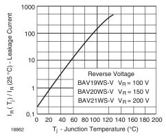
Figure 5. Leakage Current vs. Junction Temperature
