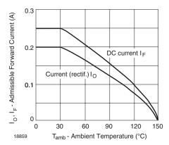
Figure 2. Admissible Forward Current vs. Ambient Temperature
