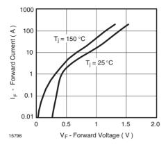
Fig. 3 Forward Current vs. Forward Voltage
