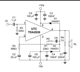
Fig. 14 Typical amplifier with split power supply
