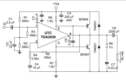
Fig. 8 Single supply high power amplifier(UTC TDA2030+BD908/BD907)
