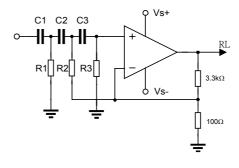
The components values calculated for fc=900Hz using a Bessel 3rd Sallen and Key structure are:  $C1=C2=C3=22nF, R1=8.2K\Omega, R2=5.6K\Omega, R3=33K\Omega.$
