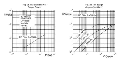
In Fig.25 The experimental results are shown for the 30W amplifier using the UTC2030A as a driver and a low-cost complementary pair. A simple RC filter on the input of the amplifier to limit the maximum signal slope(SS) is an effective way to reduce TIM.
