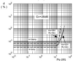
Fig.5 Two tone CCIF intermodulation distortion Po(W)
