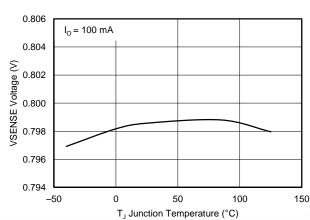
Figure 6. VSENSE VOLTAGE vs JUNCTION TEMPERATURE
