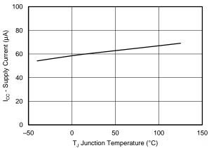
Figure 1. SUPPLY CURRENT vs JUNCTION TEMPERATURE
