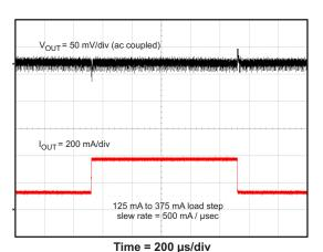
Figure 12. Loop Response, I<sub>OUT</sub> = 0.25 A
