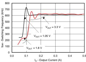
Figure 5. SWITCHING FREQUENCY vs OUTPUT CURRENT
