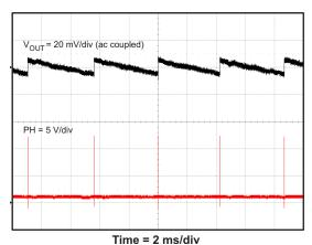
Figure 18. Output Ripple, I<sub>OUT</sub> = 0 mA
