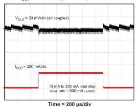
Figure 14. Transient Response, 2% to 50% Load Step
