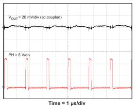
Figure 16. Output Ripple, I<sub>OUT</sub> = 500 mA
