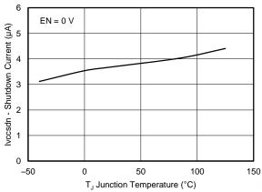
Figure 2. SHUTDOWN CURRENT vs JUNCTION TEMPERATURE
