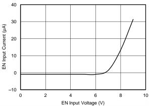
Figure 3. EN INPUT CURRENT vs EN INPUT VOLTAGE
