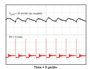
Figure 17. Output Ripple, I<sub>OUT</sub> = 30 mA
