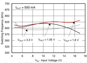
Figure 4. SWITCHING FREQUENCY vs INPUT VOLTAGE
