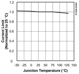
Figure 58. Internal Current Limit vs. Temperature.
