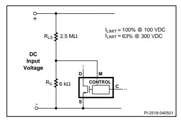
Figure 35. Current Limit Reduction with Line Voltage.
