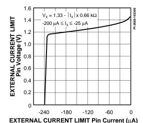
Figure 62b. EXTERNAL CURRENT LIMIT Pin Voltage vs. Current.
