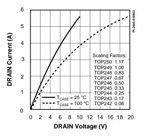
Figure 66. Output Characteristics.
