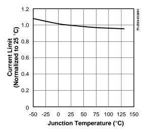
Figure 59. External Current Limit vs. Temperature with  $R_{IL}$  =12 k $\Omega$ .
