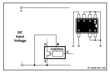
Figure 30. Three Terminal Operation (MULTI-FUNCTION Features Disabled).
