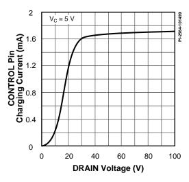
Figure 67.  $I_c$  vs. DRAIN Voltage.
