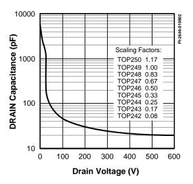
Figure 68. C<sub>OSS</sub> vs. DRAIN Voltage.
