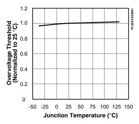
Figure 60. Overvoltage Threshold vs. Temperature.
