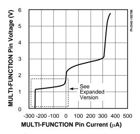
Figure 63a. MULTI-FUNCTION Pin Voltage vs. Current.
