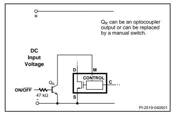
Figure 36. Active-on (Fail Safe) Remote ON/OFF.
