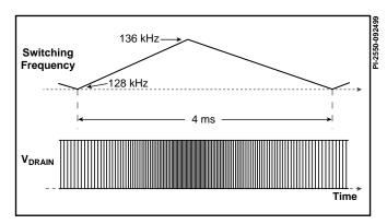
Figure 9. Switching Frequency Jitter (Idealized  $V_{DRAIN}$  waveform).
