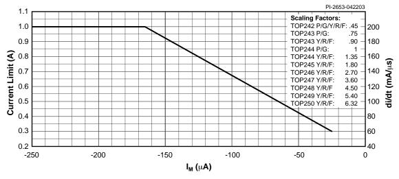
Figure 54. Current Limit vs. MULTI-FUNCTION Pin Current.
