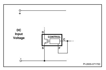
Figure 14. Half Frequency Operation (66 kHz).
