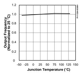
Figure 57. Frequency vs. Temperature.
