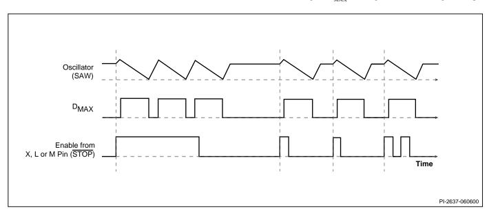
Figure 10. Synchronization Timing Diagram.
