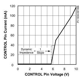
Figure 51. CONTROL Pin I-V Characteristic.
