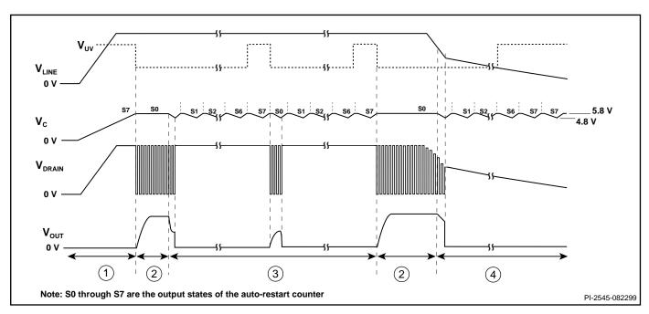
Figure 8. Typical Waveforms for (1) Power Up (2) Normal Operation (3) Auto-restart (4) Power Down.
