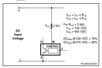
Figure 5. P/G Package Line Sense.
