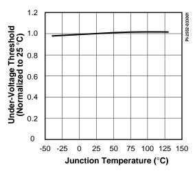
Figure 61. Under-Voltage Threshold vs. Temperature.
