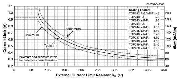
Figure 55. Current Limit vs. External Current Limit Resistance.
