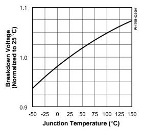
Figure 56. Breakdown Voltage vs. Temperature.
