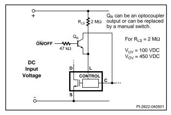
Figure 26. Active-off Remote ON/OFF with LINE-SENSE.
