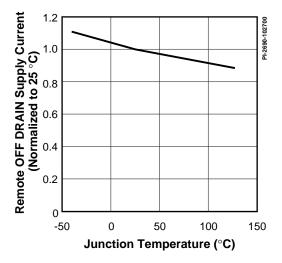
Figure 70. Remote OFF DRAIN Supply Current vs. Temperature.
