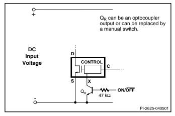
Figure 22. Active-on (Fail Safe) Remote ON/OFF.
