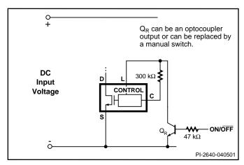
Figure 29. Active-on Remote ON/OFF.
