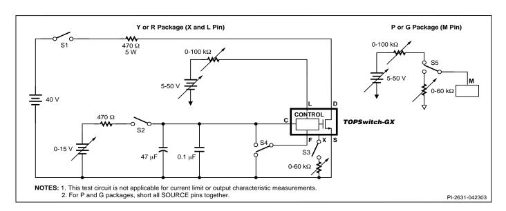
Figure 53. TOPSwitch-GX General Test Circuit.
