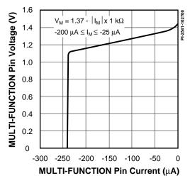
Figure 63b. MULTI-FUNCTION Pin Voltage vs. Current (Expanded).
