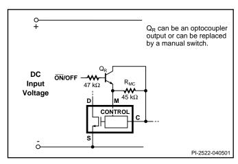
Figure 37. Active-off Remote ON/OFF. Maximum Duty Cycle will be Reduced.
