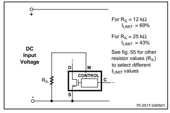
Figure 34. Externally Set Current Limit.
