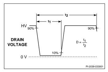
Figure 50. Duty Cycle Measurement.
