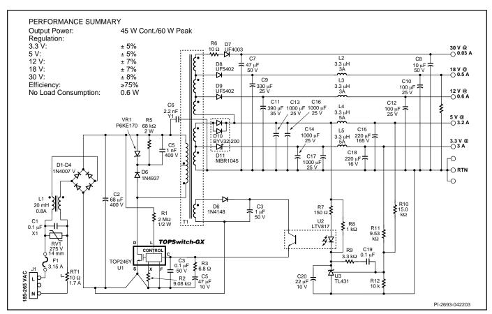
Figure 44. 60 W Multiple Output Power Supply using TOP246.
