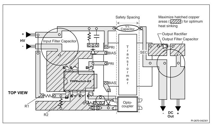
Figure 47. Layout Considerations for TOPSwitch-GX using P or G Packages.
