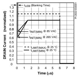
Figure 52. Drain Current Operating Envelope.
