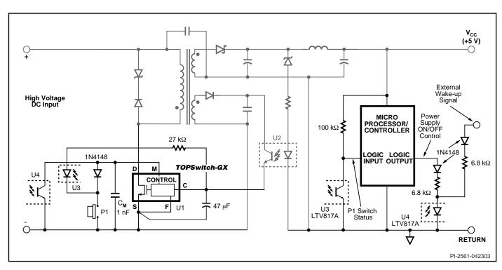
Figure 45. Remote ON/OFF using Microcontroller.
