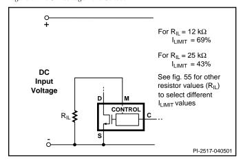
Figure 6. P/G Package Externally Set Current Limit.
