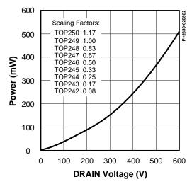
Figure 69. DRAIN Capacitance Power.
