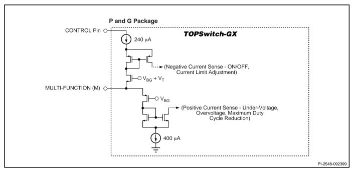
Figure 12b. MULTI-FUNCTION (M) Pin Input Simplified Schematic.
