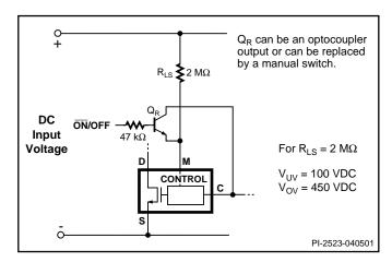
Figure 40. Active-off Remote ON/OFF with LINE-SENSE.
