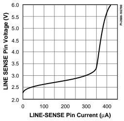
Figure 62a. LINE-SENSE Pin Voltage vs. Current.
