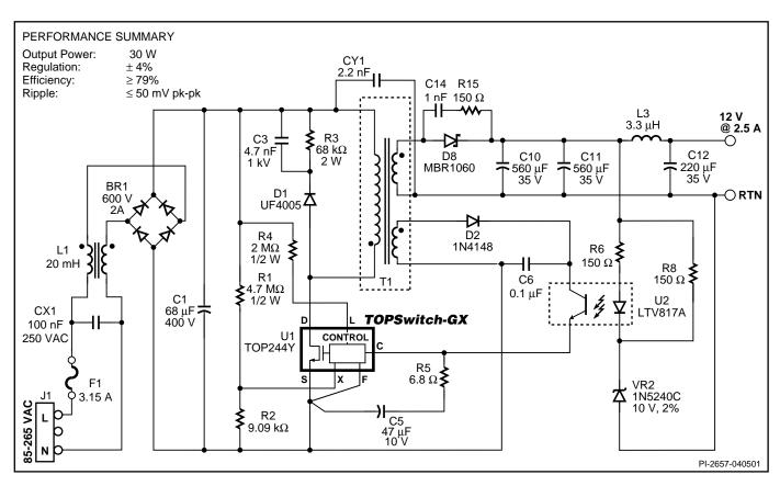
Figure 41. 30 W Power Supply using External Current Limit Programming and Line Sensing for UV and OV.
