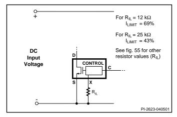
Figure 20. Externally Set Current Limit.
