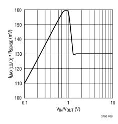
Figure 8. Load Current vs VIN/VOLIT
