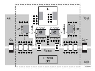
Figure 10. Switches Layout
