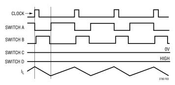
Figure 3. Buck Mode  $(V_{IN} > V_{OUT})$
