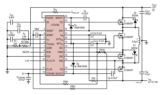
Figure 13. LTC3780 12V/5A, Buck-Boost Regulator
