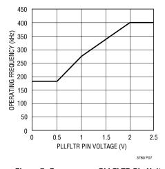
Figure 7. Frequency vs PLLFLTR Pin Voltage
