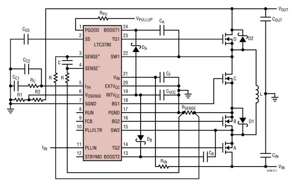
Figure 11. LTC3780 Layout Diagram
