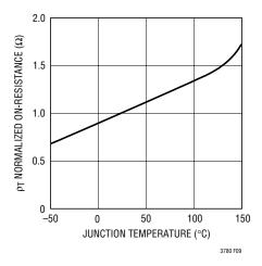
Figure 9. Normalized R<sub>DS(ON)</sub> vs Temperature
