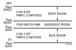
Figure 2. Operating Mode vs Duty Cycle
