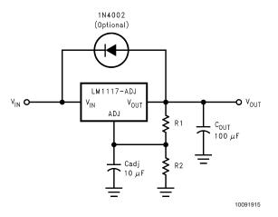
FIGURE 4. Regulator with Protection Diode
