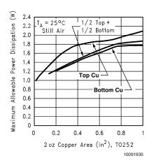
FIGURE 12. Maximum Allowable Power Dissipation vs. 20z Copper Area for TO-252
