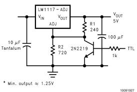
5V Logic Regulator with Electronic Shutdown\*
