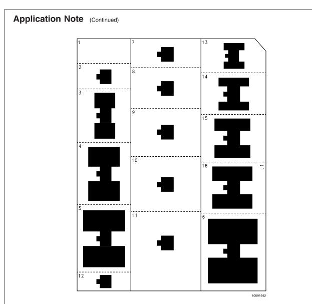
FIGURE 14. Bottom View of the Thermal Test Pattern in Actual Scale
