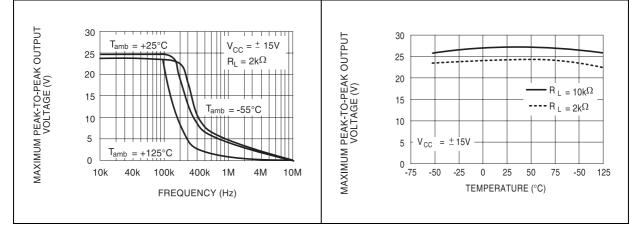
Figure 6. Maximum peak-to-peak output voltage versus load resistance
