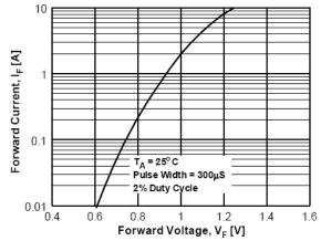
**Figure 3. Forward Voltage Characteristics**
