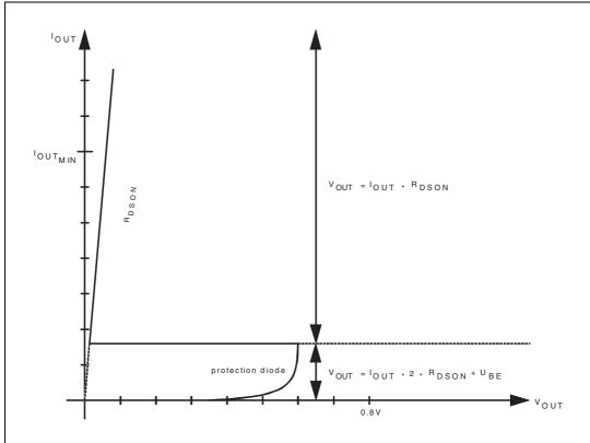
Figure 6. Output characteristics at K, LO, RX
