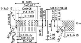
Ground area  $< \boxtimes \boxtimes :1$  to  $5\mu$ m thick solder plated>
