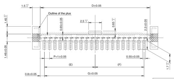
Conductive traces in this area must be covered by dielectric compound.
