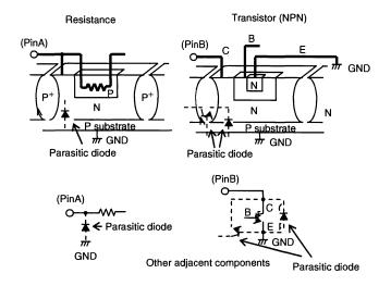
Fig-1 Simplified structure of a Bipolar IC
