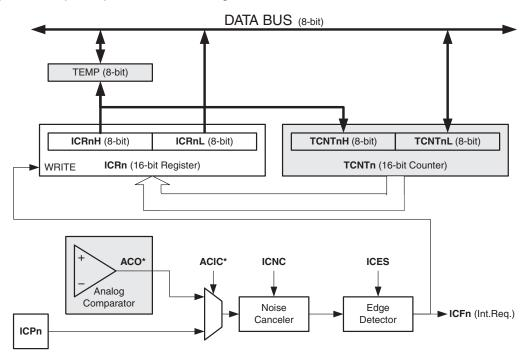
Figure 42. Input Capture Unit Block Diagram
