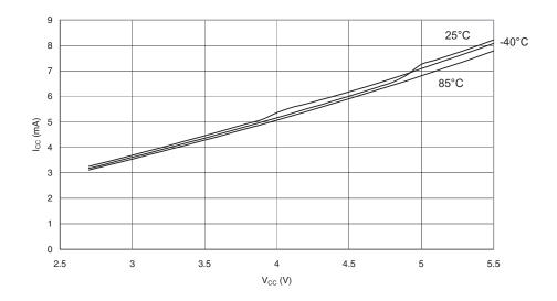
Figure 153. Active Supply Current vs. V<sub>CC</sub> (Internal RC Oscillator, 2 MHz)
