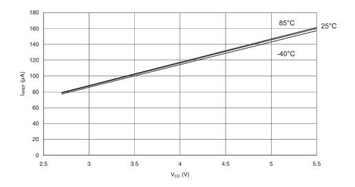
Figure 209. 32khz Tosc Current vs. V<sub>CC</sub> (Watchdog Timer Disabled)
