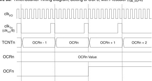
**Figure 36.** Timer/Counter Timing Diagram, Setting of OCF0, with Prescaler ( $f_{clk_l/O}/8$ )
