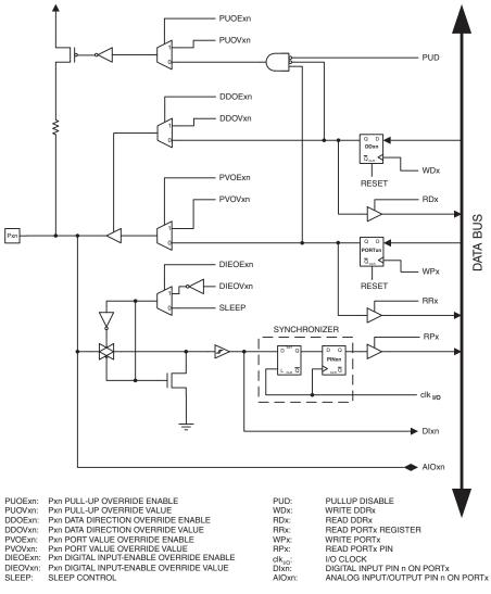
Figure 26. Alternate Port Functions<sup>(1)</sup>
