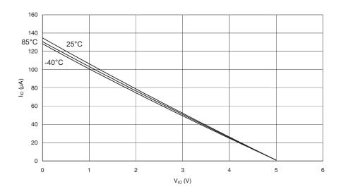
Figure 175. I/O Pin Pull-Up Resistor Current vs. Input Voltage (V<sub>CC</sub> = 2.7V)
