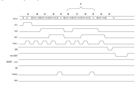
**Figure 129.** Programming the Flash Waveforms<sup>(1)</sup>
