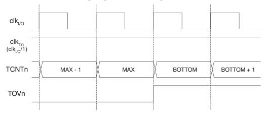
Figure 34. Timer/Counter Timing Diagram, no Prescaling
