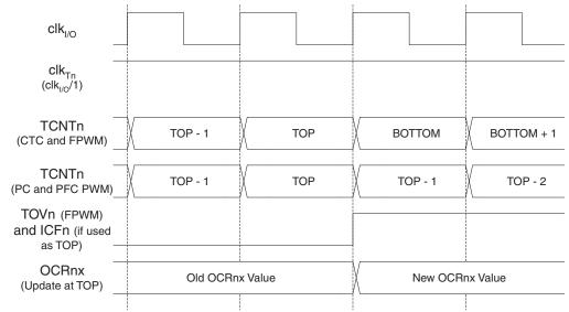
Figure 51. Timer/Counter Timing Diagram, no Prescaling
