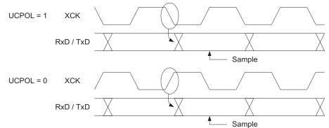
The UCPOL bit UCRSC selects which XCK clock edge is used for data sampling and which is used for data change. As Figure 71 shows, when UCPOL is zero the data will be changed at rising XCK edge and sampled at falling XCK edge. If UCPOL is set, the data will be changed at falling XCK edge and sampled at rising XCK edge.
