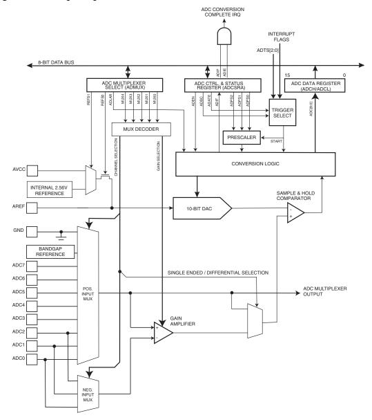
Figure 98. Analog to Digital Converter Block Schematic
