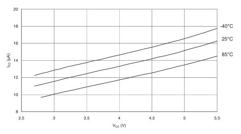
Figure 207. ADC Current vs. V<sub>CC</sub>(Aref = AVCC)
