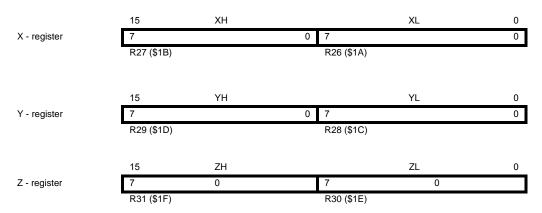
Figure 5. The X-register, Y-register, and Z-register
