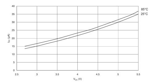
Power-Down Supply Figure 163. Power-Down Supply Current vs. V<sub>CC</sub> (Watchdog Timer Disabled) Current
