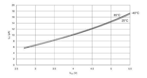
**Power-Save Supply** Figure 165. Power-Save Supply Current vs. V<sub>CC</sub> (Watchdog Timer Disabled) Current
