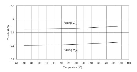
Figure 189. Bod Thresholds vs. Temperature (Bodlevel is 2.7V)
