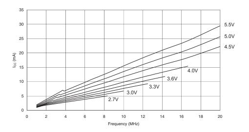
Figure 151. Active Supply Current vs. V<sub>CC</sub> (Internal RC Oscillator, 8 MHz)
