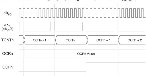
Figure 62. Timer/Counter Timing Diagram, Setting of OCF2, with Prescaler ( $f_{clk_l/O}/8$ )
