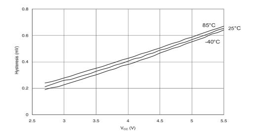
Figure 185. Reset Input Threshold Voltage vs.  $V_{CC}$  (V<sub>IH</sub>, Reset Pin Read As '1')
