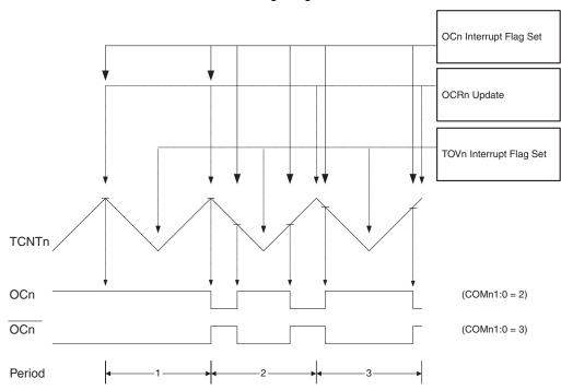
Figure 33. Phase Correct PWM Mode, Timing Diagram
