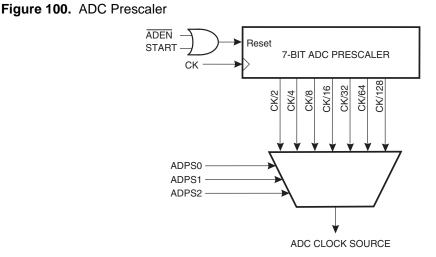
By default, the successive approximation circuitry requires an input clock frequency between 50 kHz and 200 kHz to get maximum resolution. If a lower resolution than 10 bits is needed, the input clock frequency to the ADC can be higher than 200 kHz to get a higher sample rate.
