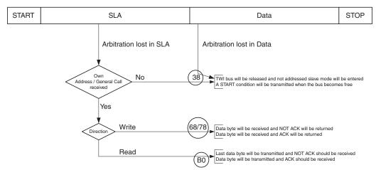
Figure 96. Possible Status Codes Caused by Arbitration
