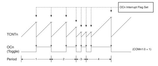
An interrupt can be generated each time the counter value reaches the TOP value by using the OCF2 Flag. If the interrupt is enabled, the interrupt handler routine can be used for updating the TOP value. However, changing the TOP to a value close to BOTTOM when the counter is running with none or a low prescaler value must be done with care since the CTC mode does not have the double buffering feature. If the new value written to OCR2 is lower than the current
