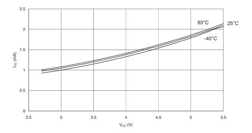
Figure 155. Active Supply Current vs.  $V_{CC}$  (32 kHz External Oscillator)
