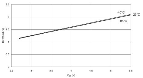
Figure 183. I/O Pin Input Threshold Voltage vs.  $V_{CC}$  (V $_{\rm IL},$  I/O Pin Read As '0')
