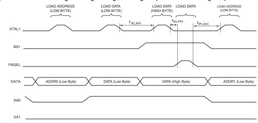
Figure 134. Parallel Programming Timing, Loading Sequence with Timing Requirements<sup>(1)</sup>
