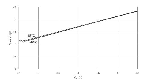
Figure 186. Reset Input Threshold Voltage vs.  $V_{CC}$  (V<sub>IL</sub>, Reset Pin Read As '0')
