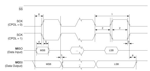
Figure 147. SPI Interface Timing Requirements (Master Mode)
