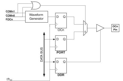
Figure 30. Compare Match Output Unit, Schematic
