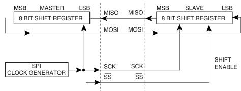
Figure 66. SPI Master-Slave Interconnection
