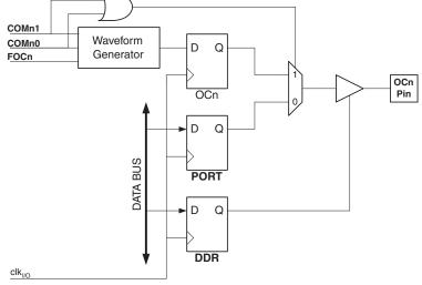
The general I/O port function is overridden by the Output Compare (OC2) from the waveform generator if either of the COM21:0 bits are set. However, the OC2 pin direction (input or output) is still controlled by the Data Direction Register (DDR) for the port pin. The Data Direction Register bit for the OC2 pin (DDR\_OC2) must be set as output before the OC2 value is visible on the pin. The port override function is independent of the Waveform Generation mode.
