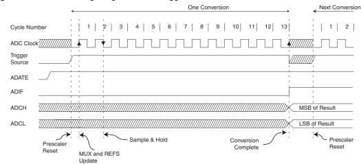
Figure 103. ADC Timing Diagram, Auto Triggered Conversion
