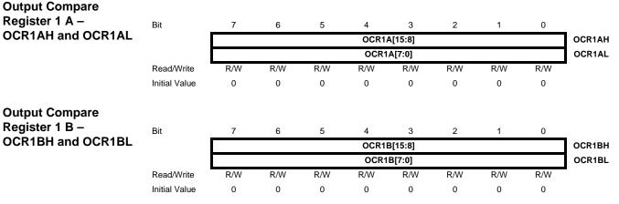
The Output Compare Registers contain a 16-bit value that is continuously compared with the counter value (TCNT1). A match can be used to generate an output compare interrupt, or to generate a waveform output on the OC1x pin.
