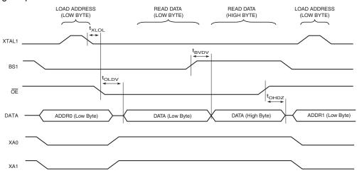
Note: 1. The timing requirements shown in Figure 133 (that is, t<sub>DVXH</sub>, t<sub>XHXL</sub>, and t<sub>XLDX</sub>) also apply to reading operation.
