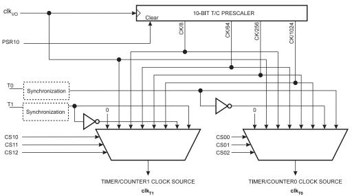
Figure 39. Prescaler for Timer/Counter0 and Timer/Counter1<sup>(1)</sup>
