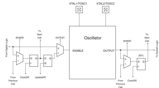
Figure 120. Boundary-scan Cells for Oscillators and Clock Options
