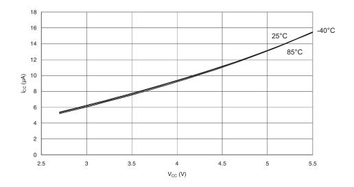
Figure 211. Programming Current vs. V<sub>CC</sub>
