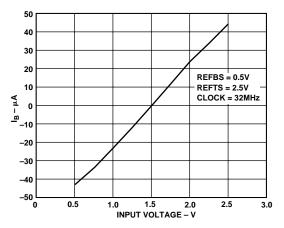
Figure 14. Input Bias Current vs. Input Voltage
