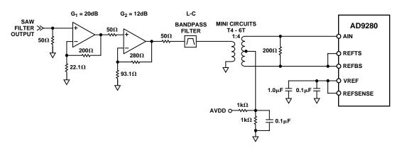
Figure 34. Simplified AD9280 IF Sampling Circuit
