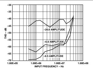
Figure 7. THD vs. Input Frequency
