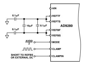
Figure 24b. Video Clamp Circuit
