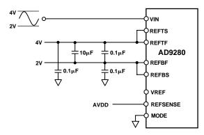
Figure 23a. External Reference—2 V p-p Input Span
