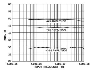
Figure 5. SNR vs. Input Frequency
