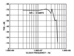
Figure 8. THD vs. Clock Frequency
