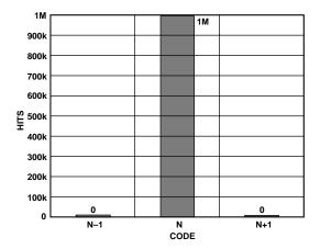
Figure 11. Grounded Input Histogram
