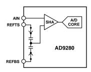
Figure 15. AD9280 Equivalent Functional Input Circuit In single-ended operation, the input spans the range,
