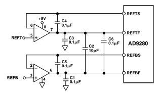
Figure 23b. Kelvin Connected Reference Using the AD9280
