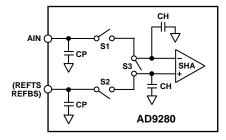
Figure 25. AD9280 Equivalent Input Structure
