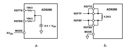
Figure 1. Equivalent Input Load
