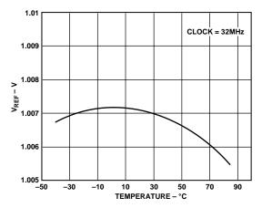
Figure 9. Voltage Reference Error vs. Temperature
