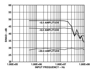
Figure 6. SINAD vs. Input Frequency
