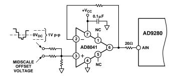
Figure 28. Bipolar Level Shift
