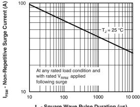
t<sub>p</sub> - Square Wave Pulse Duration (μs)
