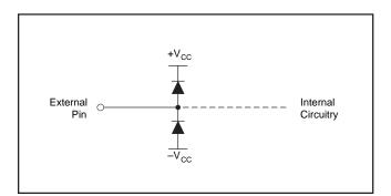
FIGURE 10. Internal ESD Protection.
