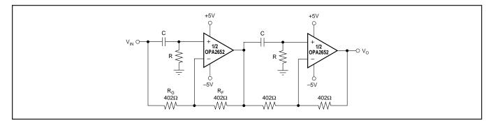
FIGURE 6. Pulse Delay Circuit.
