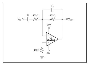
FIGURE 7. Inverting Bandpass Filter.
