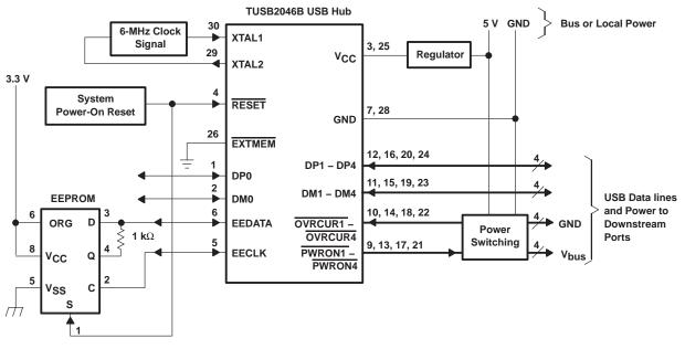
Figure 9. Typical Application of the TUSB2046B USB Hub
