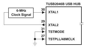
Figure 7. 6-MHz Input Clock Configuration
