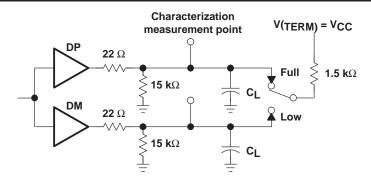
Figure 1. Differential Driver Switching Load
