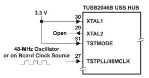
Figure 8. 48-MHz Input Clock Configuration
