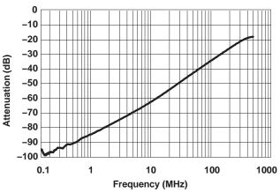
Figure 10. OFF Isolation vs Frequency
