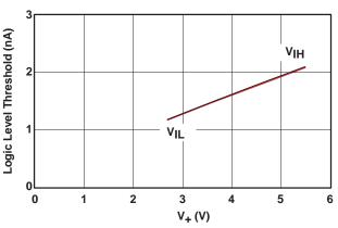
Figure 8. Logic-Level Threshold vs V<sub>+</sub>
