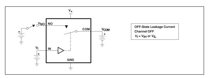
Figure 14. OFF-State Leakage Current (I<sub>COM(OFF)</sub>, I<sub>NO(OFF)</sub>)
