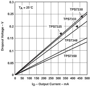
Figure 1. Dropout Voltage Versus Output Current
