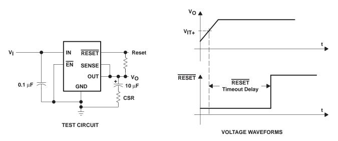
Figure 5. Test Circuit and Voltage Waveforms
