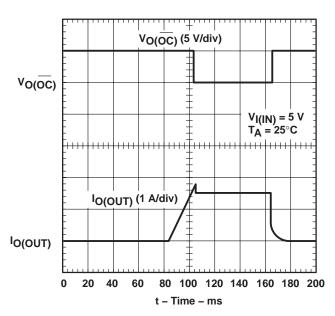
Figure 9. TPS2032, Ramped Load on Enabled Device
