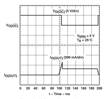
Figure 7. TPS2030, Ramped Load on Enabled Device
