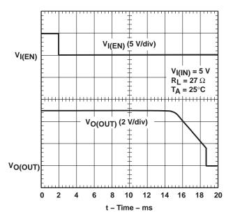
Figure 3. Turnoff Delay and Fall Time
