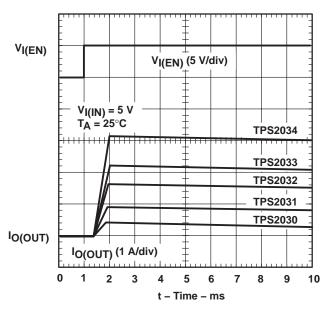
Figure 6. Device Enabled Into Short
