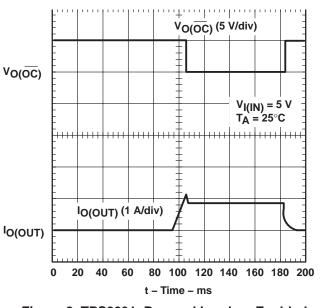
Figure 8. TPS2031, Ramped Load on Enabled Device
