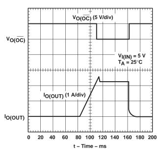
Figure 10. TPS2033, Ramped Load on Enabled Device
