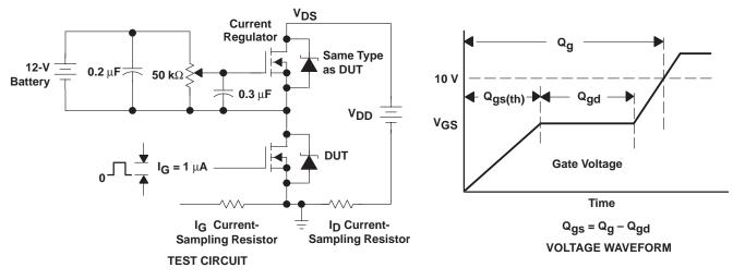
Figure 3. Gate-Charge Test Circuit and Voltage Waveform
