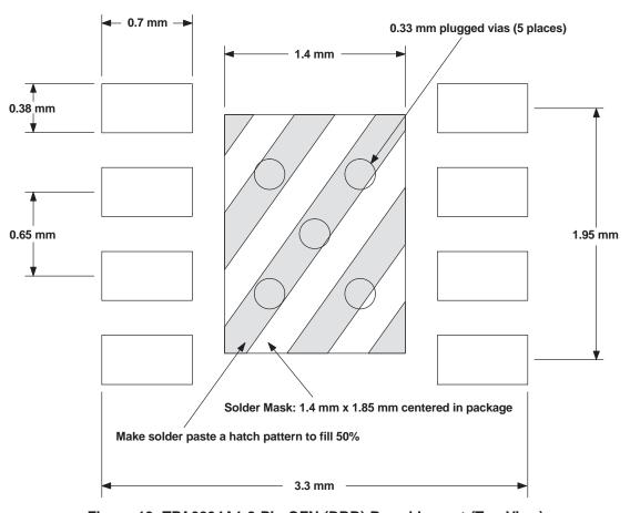
Figure 19. TPA6204A1 8-Pin QFN (DRB) Board Layout (Top View)
