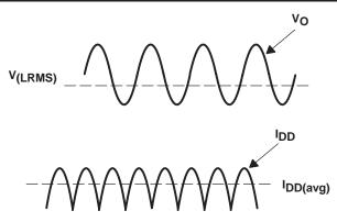
Figure 18. Voltage and Current Waveforms for **BTL Amplifiers**
