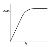
The value of  $C_l$  is important to consider as it directly affects the bass (low frequency) performance of the circuit. Consider the example where  $R_l$  is 10 k $\Omega$  and the specification calls for a flat bass response down to 100 Hz. Equation 2 is reconfigured as equation 3.
