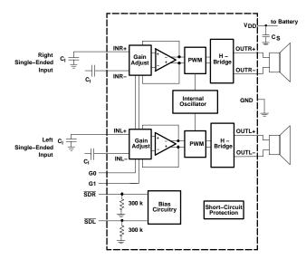
Figure 32. TPA2012D2 Application Schematic With Single-Ended Input
