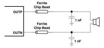
Figure 34. Typical Ferrite Chip Bead Filter (Chip bead example: TDK: MPZ1608S221A)
