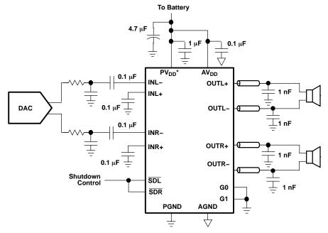
$<sup>^{\</sup>ast}$  For QFN, an additional capacitor is recomended for the second PV<sub>DD</sub> pin.
