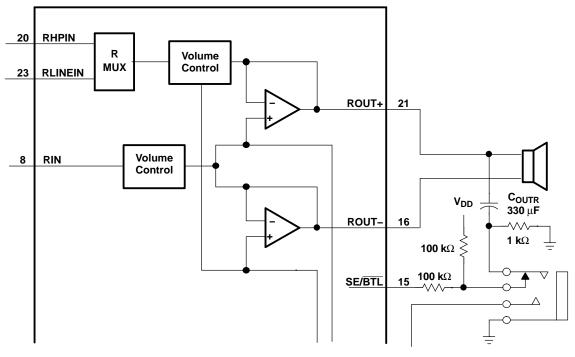
Figure 42. TPA0312 Resistor Divider Network Circuit
