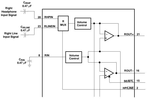
Figure 43. TPA0312 Example Input MUX Circuit
