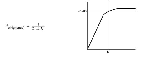
The value of C<sub>1</sub> is important to consider as it directly affects the bass (low frequency) performance of the circuit. Consider the example where Z<sub>1</sub> is 26 k $\Omega$  and the specification calls for a flat bass response down to 65 Hz. Equation 2 is reconfigured as Equation 3.
