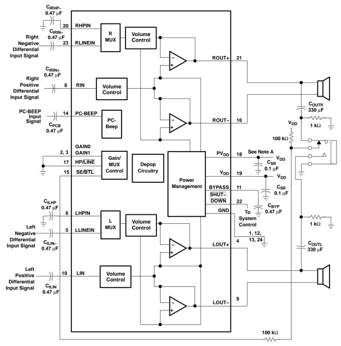
A. A  $0.1-\mu$ F ceramic capacitor should be placed as close as possible to the IC. For filtering lower frequency noise signals, a larger electrolytic capacitor of 10  $\mu$ F or greater should be placed near the audio power amplifier.
