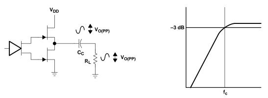
Figure 40. Single-Ended Configuration and Frequency Response
