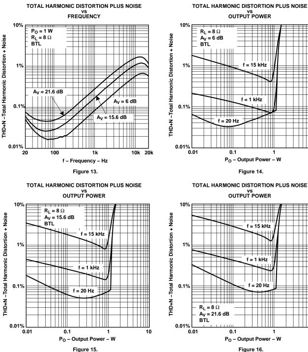
TOTAL HARMONIC DISTORTION PLUS NOISE vs OUTPUT POWER
