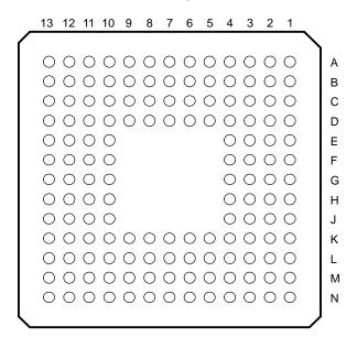
Figure 2-1. 144-Ball GGU MicroStar BGA™ (Bottom View)
