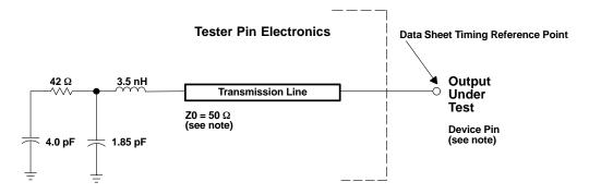
NOTE: The data sheet provides timing at the device pin. For output timing analysis, the tester pin electronics and its transmission line effects must taken into account. A transmission line with a delay of 2 ns or longer can be used to produce the desired transmission line effect. The transmission line is intended as a load only. It is not necessary to add or subtract the transmission line delay (2 ns or longer) from the data sheet timings.
