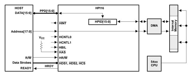
Figure 3-8. Host-Port Interface — Nonmulltiplexed Mode
