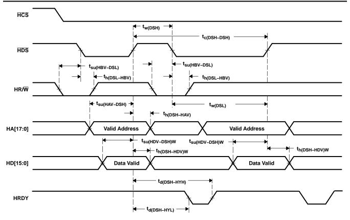
Figure 5-33. Nonmultiplexed Write Timings
