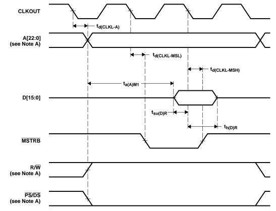
Address, R/W, PS, DS, and IS timings are all included in timings referenced as address.
