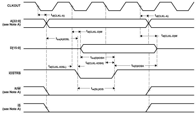
Address, R/W, PS, DS, and IS timings are all included in timings referenced as address.
