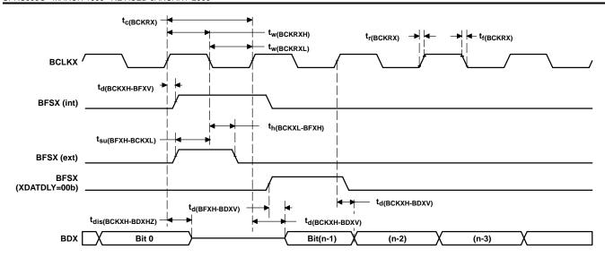
Figure 5-22. McBSP Transmit Timings
