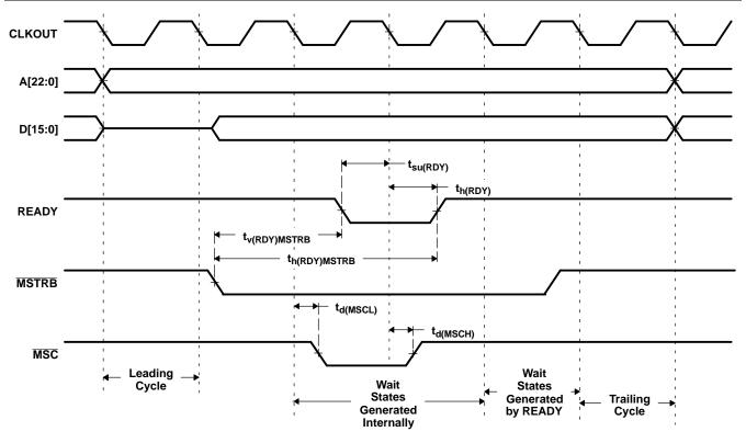
Figure 5-11. Memory Write With Externally Generated Wait States
