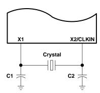
Figure 5-2. Internal Divide-By-Two Clock Option With External Crystal
