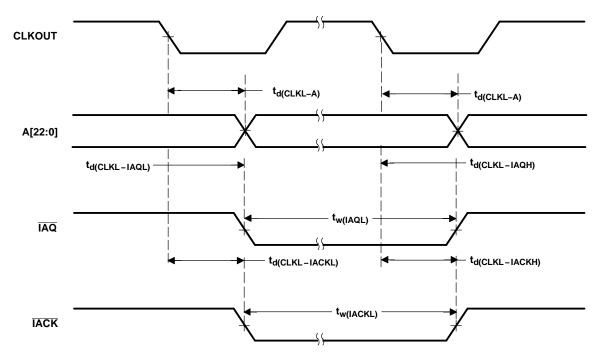
Figure 5-18. Instruction Acquisition (IAQ) and Interrupt Acknowledge (IACK) Timings
