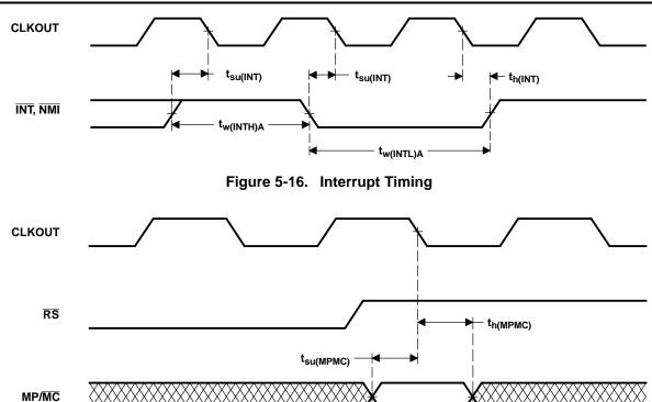
Figure 5-17. MP/MC Timing
