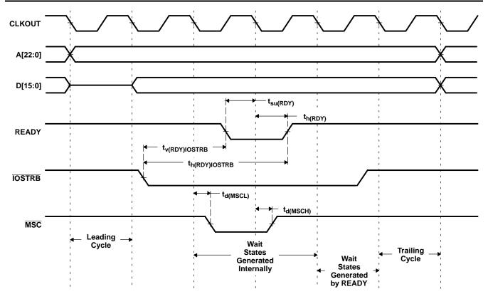
Figure 5-13. I/O Write With Externally Generated Wait States
