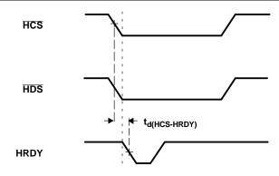
Figure 5-29. Using HCS to Control Accesses
