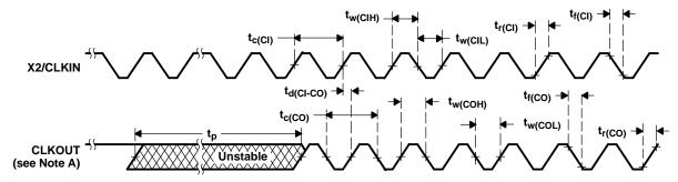
A. The CLKOUT timing in this diagram assumes the CLKOUT divide factor (DIVFCT field in the BSCR) is configured as 00 (CLKOUT not divided). DIVFCT is configured as CLKOUT divided-by-4 mode following reset.
