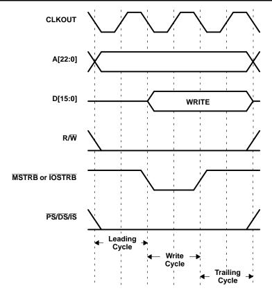
Figure 3-15. Memory Write and I/O Write Bus Sequence
