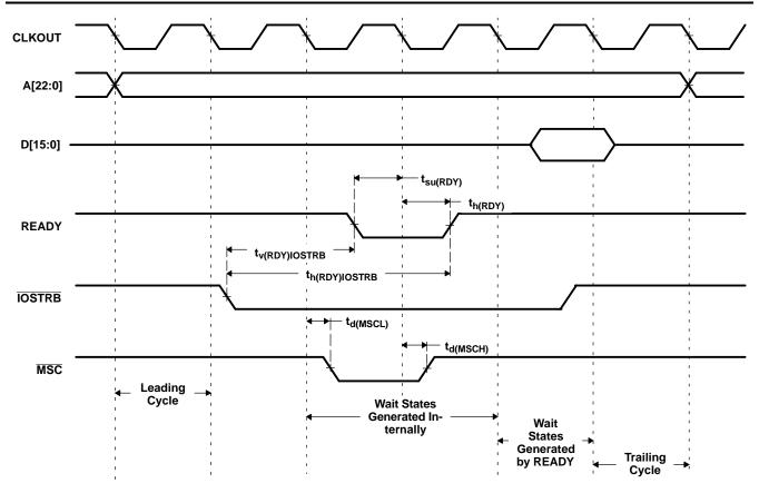
Figure 5-12. I/O Read With Externally Generated Wait States
