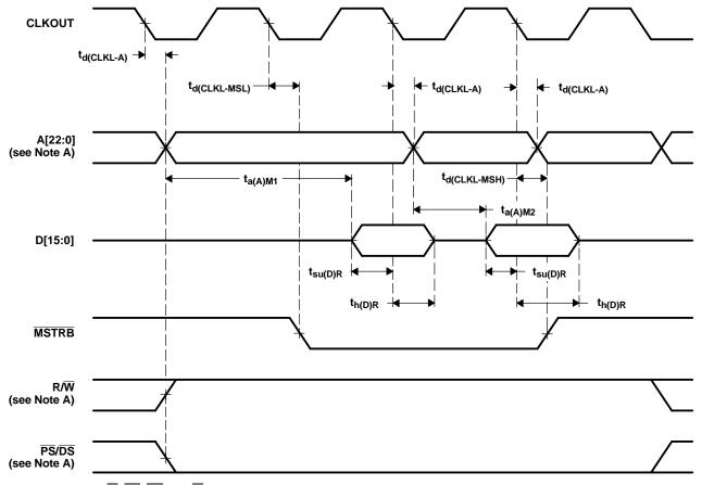
A. Address,  $R/\overline{W}$ ,  $\overline{PS}$ ,  $\overline{DS}$ , and  $\overline{IS}$  timings are all included in timings referenced as address.
