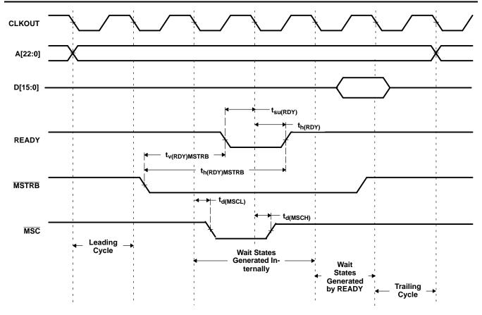
Figure 5-10. Memory Read With Externally Generated Wait States
