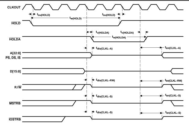
Figure 5-14.  $\overline{\text{HOLD}}$  and  $\overline{\text{HOLDA}}$  Timings (HM = 1)
