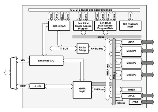
Figure 3-1. TMS320VC5416 Functional Block Diagram
