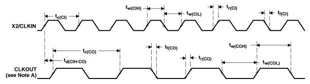
The CLKOUT timing in this diagram assumes the CLKOUT divide factor (DIVFCT field in the BSCR) is configured as 00 (CLKOUT not divided). DIVFCT is configured as CLKOUT divided-by-4 mode following reset.
