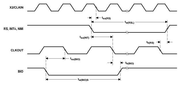
Figure 5-15. Reset and BIO Timings
