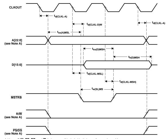
A. Address,  $R\overline{W}$ ,  $\overline{PS}$ ,  $\overline{DS}$ , and  $\overline{IS}$  timings are all included in timings referenced as address.
