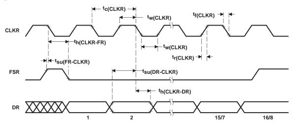
Figure 16. Serial-Port Receive Timing
