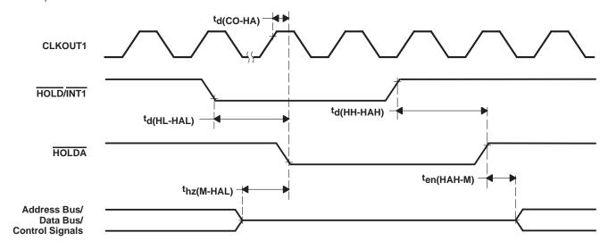
Figure 15. External DMA Timing
