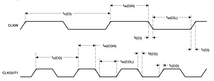
Figure 8. CLKIN-to-CLKOUT1 Timing With PLL (Enabled)
