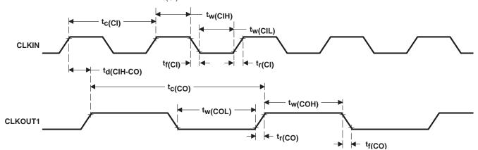
Figure 7. CLKIN-to-CLKOUT1 Timing Without PLL (using +2 clock option)
