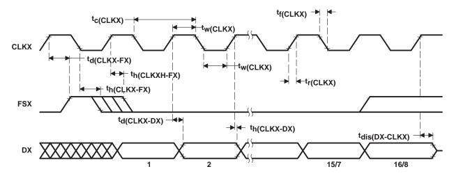
Figure 17. Serial-Port Transmit Timings
