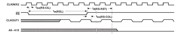
Figure 13. Reset Timing
