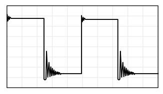
(b)  $C_L = 260 \text{ pF}, R_L = NO \text{ LOAD}$
