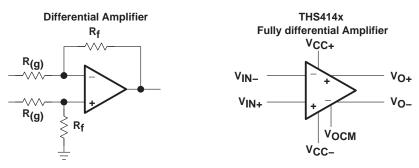
Figure 27. Differential Amplifier Versus a Fully Differential Amplifier
