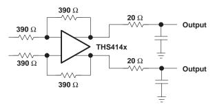
Figure 25. Driving a Capacitive Load
