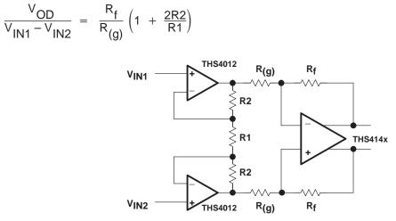
Figure 32. Instrumentation Amplifier
