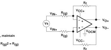
Note: For proper operation, maintain symmetry by setting  $R_{f1} = R_{f2} = R_{f}$  and  $R_{(g)}1 = R_{(g)}2 = R_{(g)}$  $\Rightarrow A = R_{f}/R_{(g)}$
