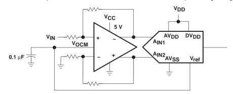
Figure 23. Fully Differential Amplifier Using a Single Supply
