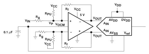
Figure 24. Circuit With Improved Common-Mode Input Voltage
