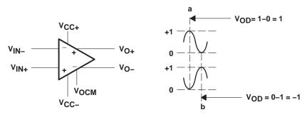
Figure 31. Fully Differential Amplifier With Two 1-VPP Signals
