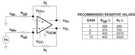
Figure 30. Single In With Differential Out
