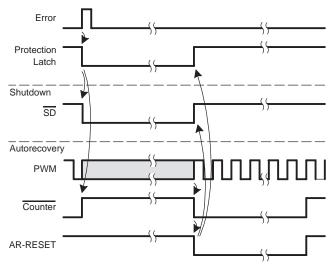
Figure 10. Autorecovery Function Latching Shutdown on All Errors (PMODE1)
