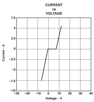
NOTE A: Typical current versus voltage curve was derived using the IEC 1.2/50-µs surge waveform.
