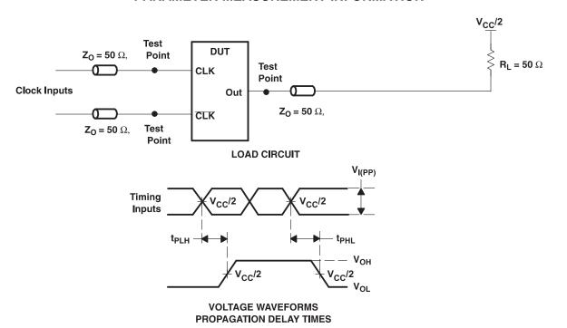
Figure 1. Output Load For Production Test
