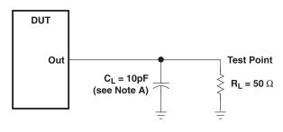
LOAD CIRCUIT LOW-TO-HIGH SLEW-RATE MEASUREMENT
