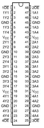
The device can be used as four 4-bit buffers, two 8-bit buffers, or one 16-bit buffer. It provides true outputs and symmetrical active-low output-enable (OE) inputs.
