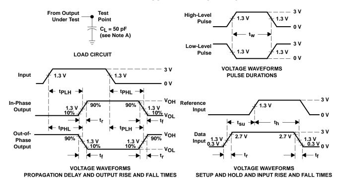
NOTES: A. C<sub>L</sub> includes probe and test-fixture capacitance.
