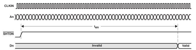
Figure 8. Enable Time Waveforms
