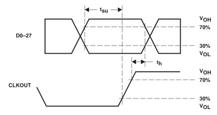
Figure 5. Setup and Hold Time Measurements
