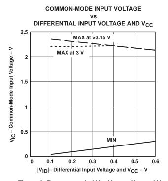
Figure 3. Recommended  $\rm V_{IC}$  Versus  $\rm V_{ID}$  and  $\rm V_{CC}$
