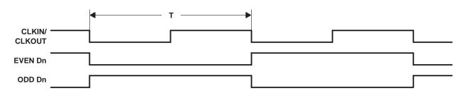
Figure 4. Worst-Case Power Test Pattern
