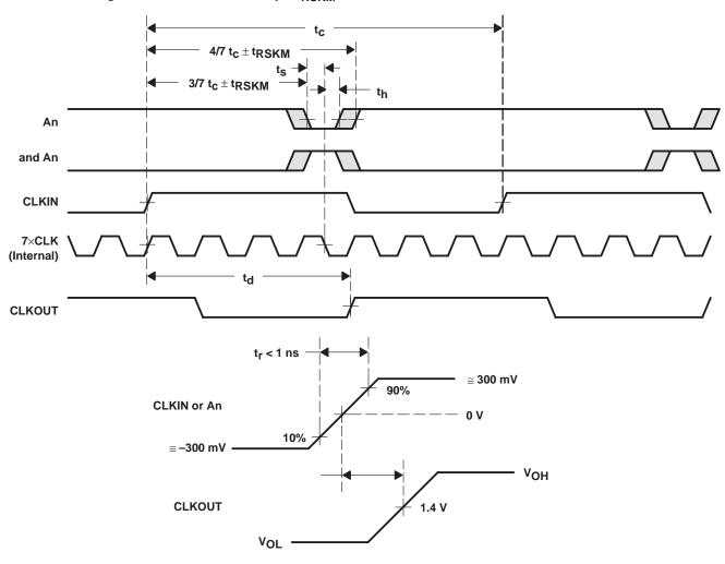
Figure 6. Receiver Input Skew Margin and t<sub>d</sub> Definitions
