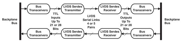
Figure 13. Virtual Backplane Transceiver
