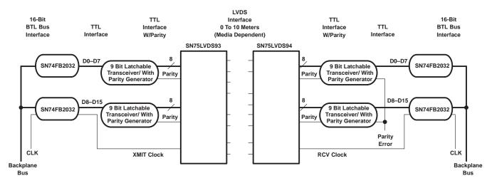
Figure 12. 16-Bit Bus Extension With Parity
