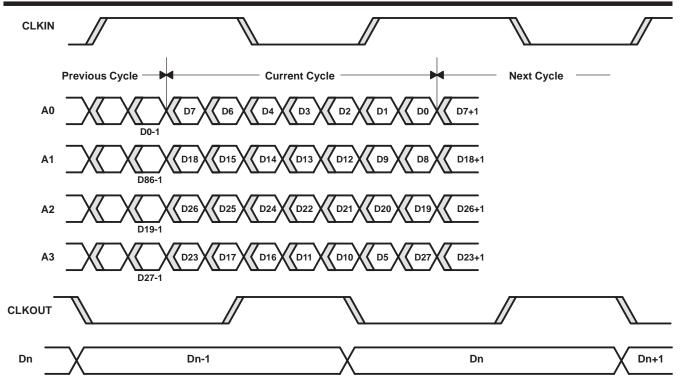
Figure 1. SN65LVDS94 Load and Shift Sequences
