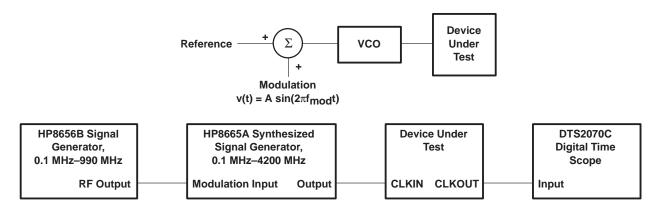
Figure 7. Output Clock Jitter Test Setup
