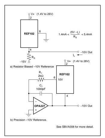
FIGURE 6. -10V Reference Using a) Resistor or b) OPA227.
