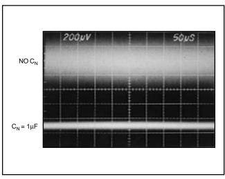
FIGURE 5. Effect of 1µF Noise Reduction Capacitor on Broadband Noise (f<sub>-3dB</sub> = 1MHz)
