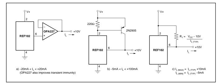
FIGURE 7. +10V Reference With Output Current Boosted to: a) ±20mA, b) +100mA, and c) I<sub>L (TYP)</sub> +10mA, -5A.
