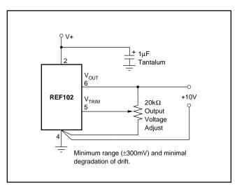
FIGURE 3. REF102 Optional Output Voltage Adjust.
