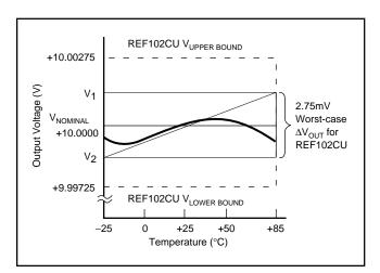
FIGURE 1. REF102CU Output Voltage Drift.
