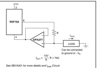
FIGURE 10. Positive Precision Current Source.
