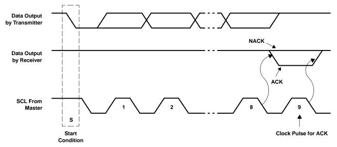
Figure 7. Acknowledgment on the I<sup>2</sup>C Bus
