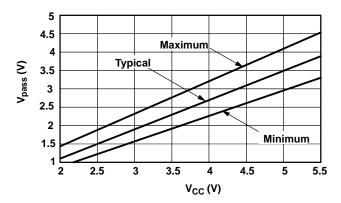
Figure 3. V<sub>pass</sub> Voltage vs V<sub>CC</sub>
