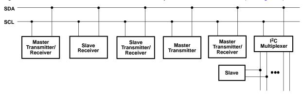
Figure 6. System Configuration
