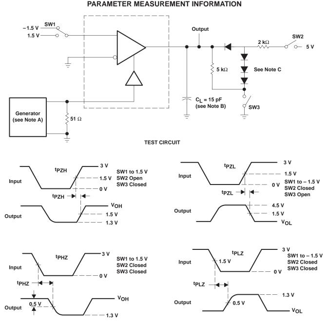
NOTES: A. The input pulse is supplied by a generator having the following characteristics: PRR  $\leq$  1 MHz, duty cycle = 50%, t<sub>r</sub>  $\leq$  6 ns, t<sub>f</sub> ≤ 6 ns.
