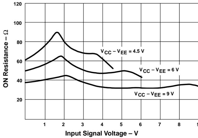
Figure 8. Typical ON Resistance vs Input Signal Voltage
