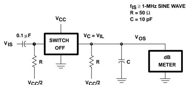
Figure 6. Switch OFF Signal Feed-Through Test Circuit
