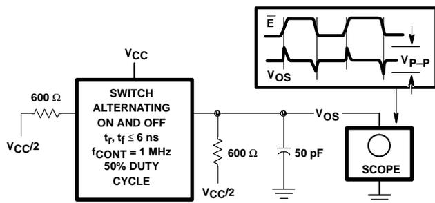
Figure 5. Control to Switch Feed-Through Noise Test Circuit
