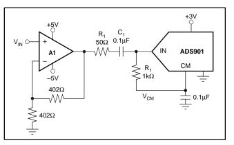
FIGURE 2. AC-Coupled, Single-Ended Interface Circuit.
