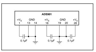
FIGURE 8. Recommended Bypassing for Analog Supply Pins.
