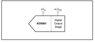
FIGURE 7. Independent Supply Connection for Output Stage.
