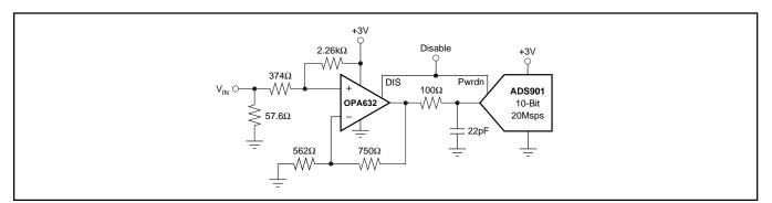
FIGURE 4. DC-Coupled Interface Circuit for +3V Single-Supply Operation.
