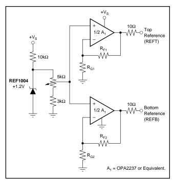
FIGURE 6. Precise Solution to Supply External Reference Voltages.
